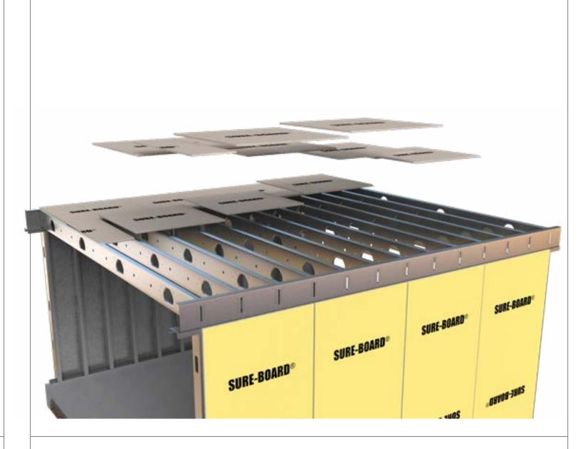
4-foot panels with 20-gauge thick hotdipped galvanized steel sheet adhered to a magnesium oxide substrate for a one-step installation that not only acts as a sub-floor but also provides a proven solution for shear.
